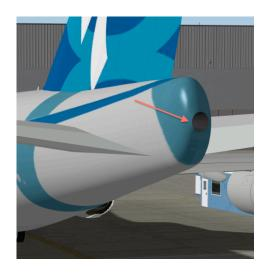
The location of the APU is in the aircraft tailcone, and its exhaust is shown in the illustration above (see arrow).
