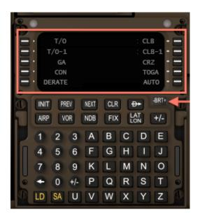
After activation, the thrust limit page appears on the CDU to select the thrust mode using the LSKs on either side of the CDU display. The modes are described as follows:
