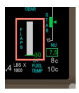
The flap position is also displayed on the Upper EICAS. Leading edge and trailing edge flaps move together according to system logic, so the same handle operates both sets of flaps as required. The flap setting is shown in magenta while the flaps are in movement and turns green when the selected flap position is reached.
