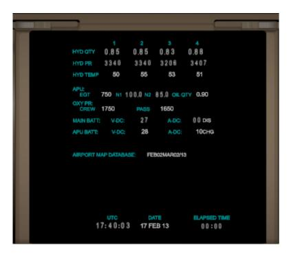
The status synoptic on the Lower EICAS provides a means to monitor the APU's status by indicating its N1 and N2 percentages. There are also status messages on the Upper EICAS associated with operation of the APU.
