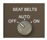
Activating the SEAT BELTS knob also triggers a chime that can be used to alert flight attendants during various phases of flight.
