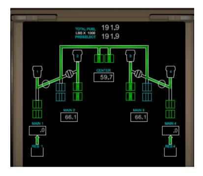
The fuel quantity in each tank is shown on the fuel synoptic, which can be displayed on the Lower EICAS.
