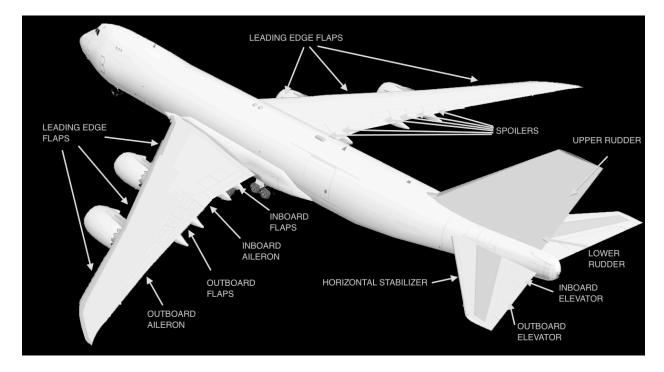
Most of these flight controls and their operation is replicated on the SSG 747-8. The flight controls synoptic is implemented as well, and can be selected on the Lower EICAS. The synoptic display shows the position of the various flight controls, including the primary flight controls, stabilizer trim and the spoilers.
