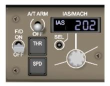
The MCP autothrottle controls also include a small SEL button that allows switching from Indicated Air Speed (IAS) to Mach Number (MACH) for the MCP speed window. Typically speeds are flown in terms of MACH above transition altitude (where the Flight Levels start) and in IAS below it.
