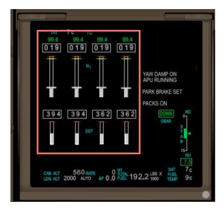
The displays within the red box above show the primary engine indications, these include (from top to bottom):
