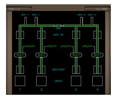
The electrical system synoptic that is accessible on the Lower EICAS is mostly cosmetic. It shows a representative display of all generators working, and it will show if the engine-driven generator bus ties are open or closed.
