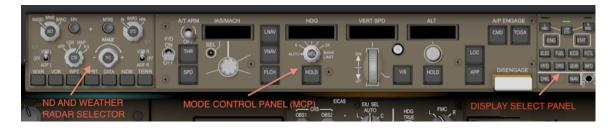
The Mode Control Panel (MCP) includes the following controls and indicators:
