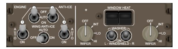
Ice and rain protection functions that can be selected on the SSG 747-8 overhead include:
