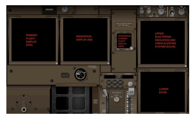
They forward panel is composed of the following displays and controls:
