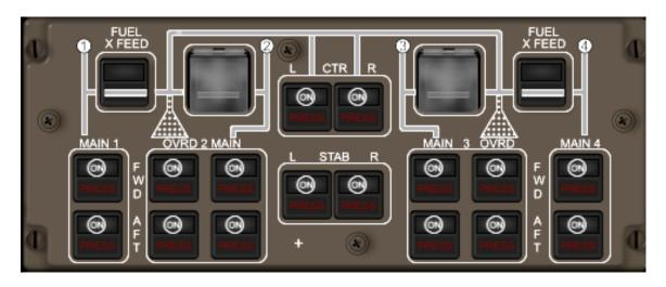
Fuel tank pumps are turned on and off with buttons on the overhead panel. Crossfeeds (X FEED) are non functional on the SSG 747-8 overhead panel.
