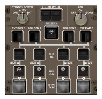
The overhead electrical panel allows for the switching of the battery on and off, as well as the bus ties to connect the engine-driven generators to the main electrical busses. The APU Generators (1 and 2) and engine Generator Controls (GEN CONT) can also be selected. This system is greatly simplified compared to the real 747-8, and the other buttons on the panel are inoperative.
