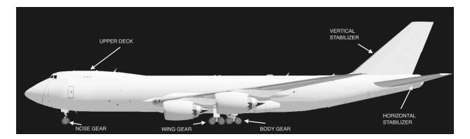
Note that the engines are numbered 1 to 4 starting from left to right of the aircraft. Also, in logical fashion, the wing gear are mounted under each wing, while the body gear are mounted on the lower fuselage body. The main gear tilt down while the body gear rotates left and right to aid in turning while taxiing. The nose gear also turns, although through a much wider range than the body gear.
