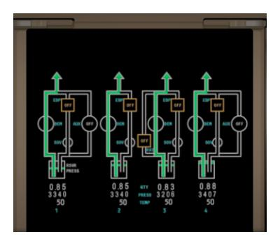
In the SSG 747-8, the hydraulic system synoptic that is selectable on the Lower EICAS is only cosmetic and shows how the display would look in normal flight operations with all hydraulic systems active. The only value that is active on the synoptic page is the hydraulic pressure (middle row of numbers).
