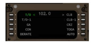
On the ground you can only select the T/O, and GA modes. If you select a T/O mode, the thrust limit mode will be a fixed value. However, if you select the DERATE mode it will assume a thrust limit based in the actual Outside Air Temperature (OAT). The thrust limit value typically will decrease with a decrease in OAT.
