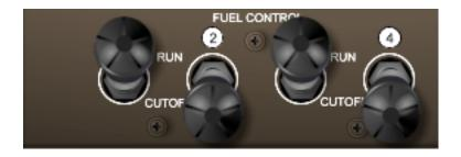
There are 4 fuel control switches located in the aisle stand portion of the SSG 747-8 panel, one switch for each engine as numbered.
