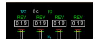
The pilots have an indication on the Upper EICAS that each individual engine is in reverse by the "REV" indication above the N1 tape white boxes.
