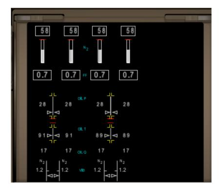
The secondary engine synoptic is accessed on the Lower EICAS, and shows the following information for each engine:
